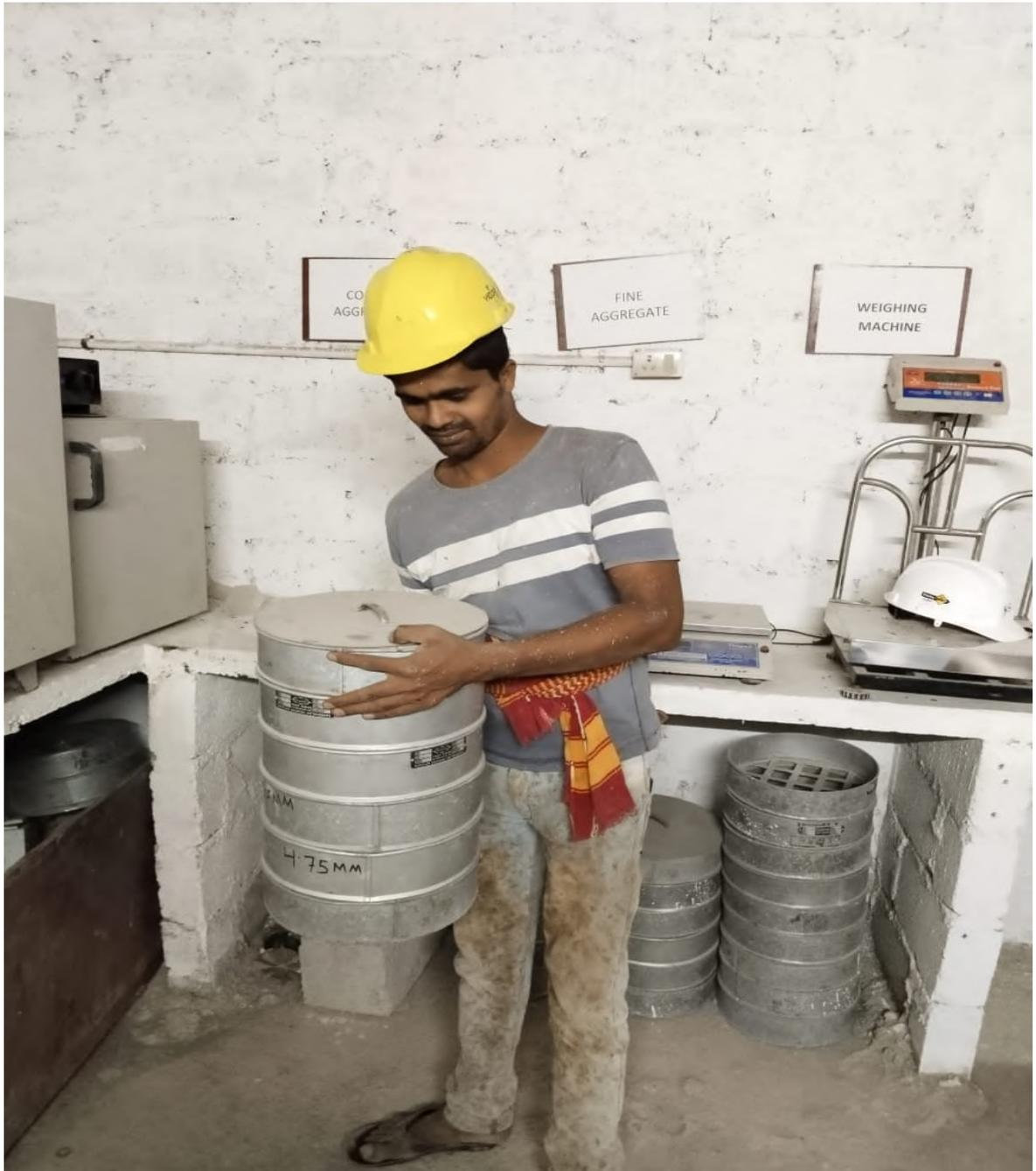
**Fine Aggregate Sieve Analysis Testing**
