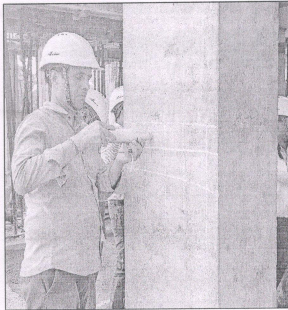
Figure 5: Typical view of Rebound Hammer Test in Progress
